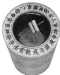
Figure 1 Boussole liquide chinoise
